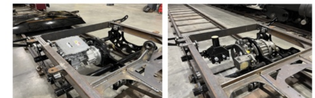
DM Drive Truck (Electric motor/inverter and gear reduction system)
