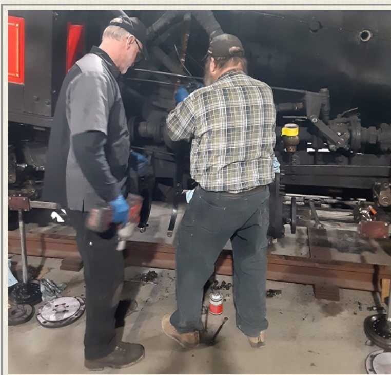
Installing New Parts: Allen Haggett (L) & Paul Forbes (R) working on No. 9's cylinder cock control mechanism. (2025) - Cookie Sodergren photo
