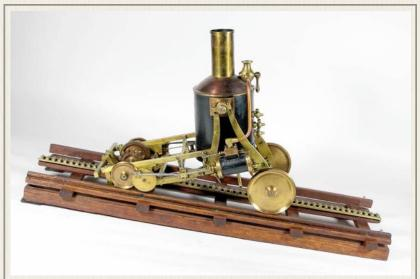
end and the boiler tilted accordingly. Unless I'm mistaken, it is currently displayed facing the wrong direction. I'm assuming whoever last modified it was more familiar with conventional steam locomotives where the cylinders face rear. The other interesting thing is that it shows Marsh's gripping mechanism *(below)*, which
