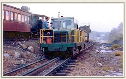
can be extended to support a walkway or to use as a boom for handling heavy material. The cab provides full head room with plenty of window space for good visibility.
