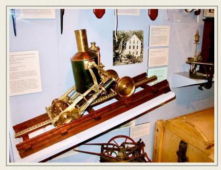
locked the cog to the rack, meaning it could never disengage.
