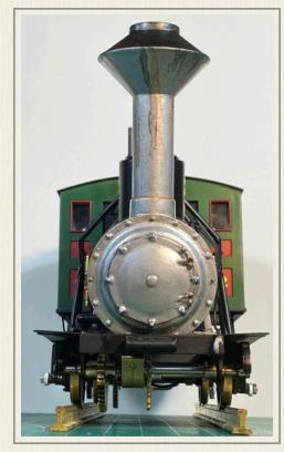
photos with lasercut brass frames and custom lost wax investment casts for the wheels and fly-cranks, while the tender tank, cab and boiler are a combination of ABS 3D printed parts, Styrene scratch building and lasercut acrylic. Currently I only have a
